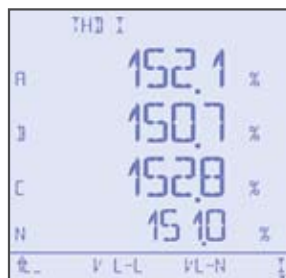
Current total harmonic distortion display
